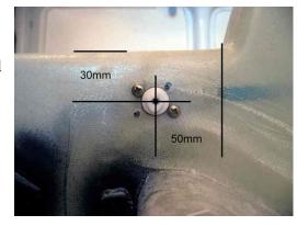
screw holes, which will be visible through the fibreglass, then remove the fuel tap and drill the holes. Pre-fit the fuel tap with the two screws and then remove the tap and set it aside.
