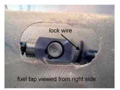
Fit the fuel line and tap assembly: cover the ends of both fuel lines to prevent foreign objects from entering by using masking tape over the ends and then insert the red fuel line end into the console through the access hole in the right-hand side and feed the red fuel line down and back towards the rear of the fuselage and into the lower longitudinal rib along the rear floor.
