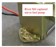
Mount the electric fuel pump to the fuselage on the right of the longitudinal rib as shown on the drawing on the previous page, using countersunk M4 screws and Tinnerman washers going through into the previously fitted captured nuts and tighten the nuts to safety.
