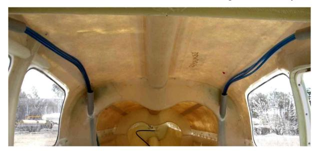
Route each fuel line around the front of the opening in the rear cabin step and leave enough length to connect to the header tank fittings, leave 500mm of free length outside of the upper fuselage. Remove the fuel lines and use each one as a measure to cut two more fuel lines of each length for each side. Label the lines as "Left" or "Right" (the shorter lines will be the "Left" set) and coil and store in a bag for later use.
