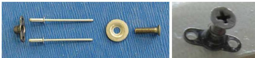
Use the captive nut itself as a jig to drill the rivet holes as shown at above right – thread the screw part way through the captive nut from the back and fit the exposed end of the thread into the hole in the fuselage, then drill the 2 x 3/32" rivet holes.
