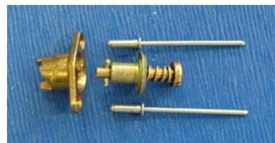
Countersink the holes in the bottom cowl enough to allow the Tinneman washers to seat snugly. Do not countersink the holes in the top cowl, just deburr them.
