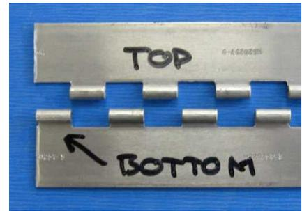
Assemble each hinge pair by sliding the long hinge pin through the full length of the hinge. Note that the hinge pin is much longer than the hinge – do **not** trim the hinge pin to length! The extra length will be used when the hinge pin is fitted through from the door jamb and into the hinge later in this task. Put a cloth tape flag on the exposed end of the hinge pin to prevent possible accidents.
