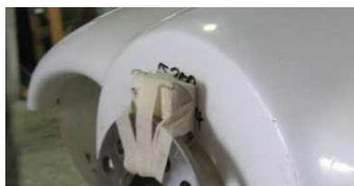
In this step we will need to make up a spacing jig (shown at left) that will keep the front of the top cowl 20mm behind the propeller flange and 15mm above and centred on the propeller shaft extension, plus a 3mm spacer on top of each ram air duct. Wooden blocks cut to size are fine for the purpose.
