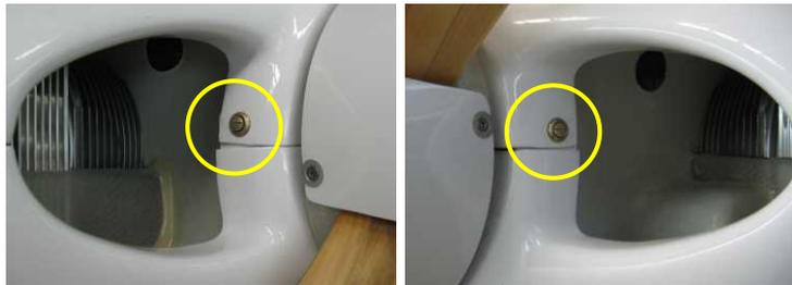
Starting with the bottom cowl, remove one 6G stainless steel screw at a time and drill the hole out to 3/16", then drill the 3 holes in the top cowl to 5/16".
