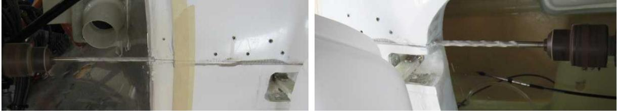
Refit the bottom cowl to the fuselage and hold the hinge in against the joggle then mark a line beside the firewall and directly behind the hinge. Drop the cowl and drill a  $\frac{1}{4}$ " hole at this point as shown above left: it will be just inside of the fuselage skin.
