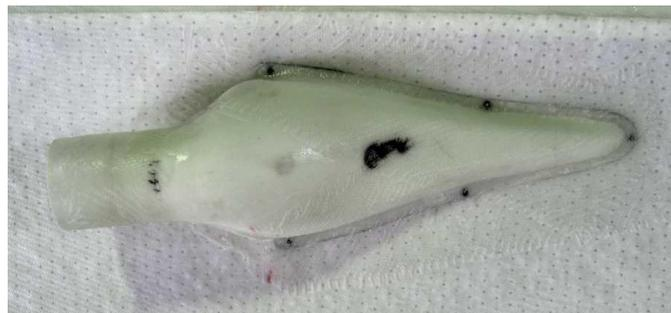
When the Araldite/flock has cured, heat and remove the screws, mix a small batch of resin and apply a single layer of AF303 glass fibre cloth on the inside of the cowl over both sides and across the rear of the scoop. Leave overnight to cure.
