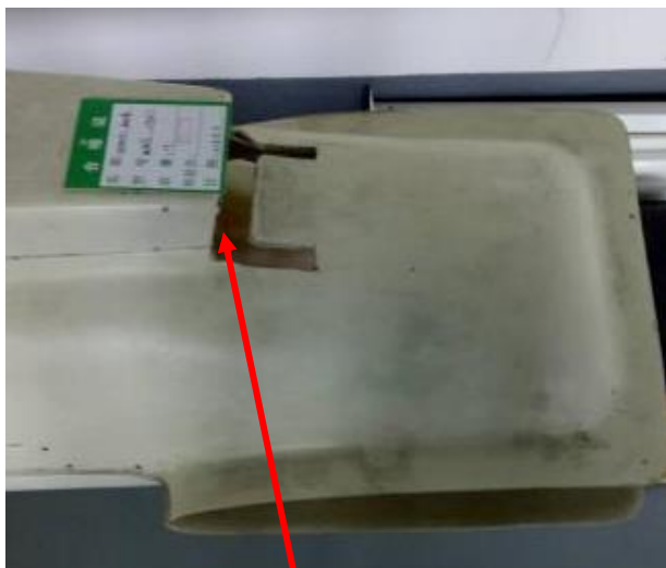
Fin post is integral with fuselage moulded stub
