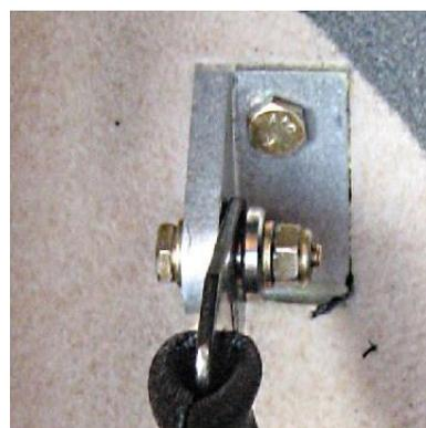
seatbelt fitting, then the heavy flat washer (from the "*Seatbelts*" card) and a plain washer then the Nyloc nut.
