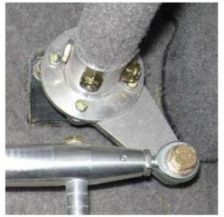
Refit the inner flap drive arm with the AN3 bolts, flat washers and Nyloc nuts and tighten the nuts to safety. Fit the outer flap drive arms to each end of the flap shaft and secure each with an AN3 bolt and Nyloc nut as shown at right. Tighten the nuts to safety.
