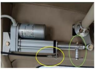
Screw the "L" shaped bracket or the Straight bracket to the bottom of the motor assembly with a countersunk screw (circled in yellow above), then drop the AN3-16A bolt down through the actuating shaft and add the 3 spacers and the 2 retaining nuts (circled in green above).
