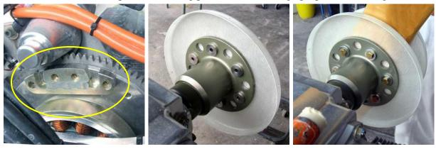
Turn the engine so that one set of flywheel magnets are at the top (circled above left). This will ensure that the propeller will stop in a horizontal position. Fit the guide bushes from the back of the propeller flange and fit the rear spinner mounting plate over them with the cupped face towards the rear. Fit the propeller so that the upper blade is closest to the 11 o'clock position when viewed from the front of the engine. Tap the bolts through with a soft hammer.
