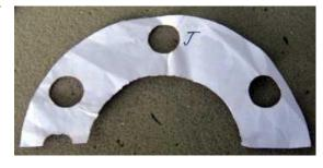
Add more shims if required. Note that a shim cut from a manila folder will correct a 2.5-3mm tracking error. Make fine adjustments as described next:
