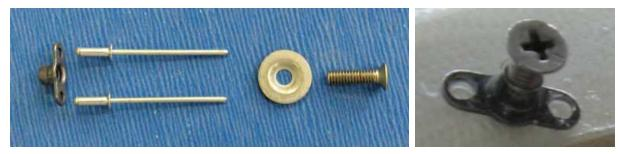
Countersink the rivet holes just enough to make a countersunk 3/32" rivet sit flush and fix the captive nuts in place and then enlarge the 5/32" holes in the mounting plates to 3/16" to provide clearance for the screw threads.
