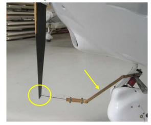
**Coarse adjustment**: if the difference between blades is greater than 1 to 1.5mm then a shim will need to be made and placed between the propeller and the propeller flange.
