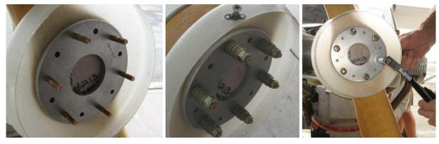
Fit the front spinner mounting plate with the cupped face towards the front, followed by the machined aluminium mounting plate.
