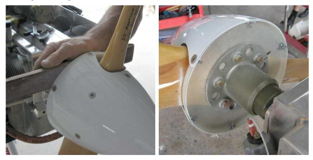
Use a long sanding block to sand the rear mounting plate flush with the rear of the spinner.
