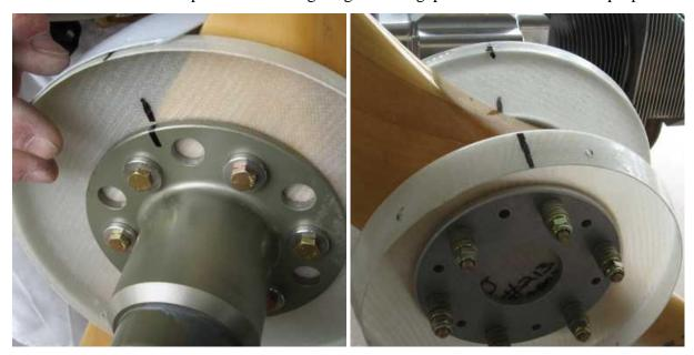
When the mounting position has been decided, mark each component with a permanent marker as shown above so that if there is any need to remove the spinner or propeller all the parts can be refitted in the same position relative to each other.
