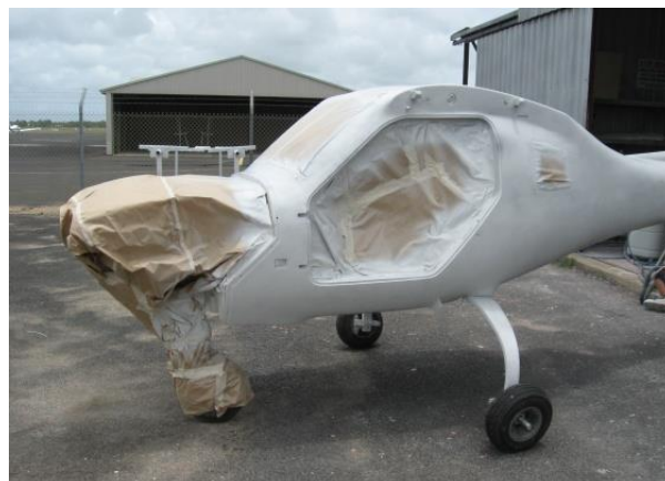
Masked and undercoated J170 fuselage
