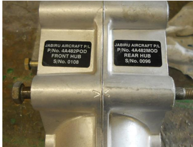
Figure 4 - Propeller hub indexing arrows
