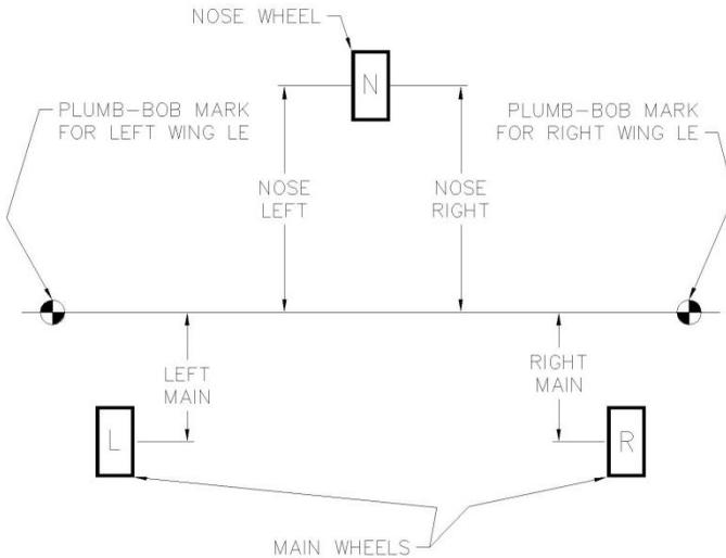
Figure 6.1.1 – Weighing Aircraft
