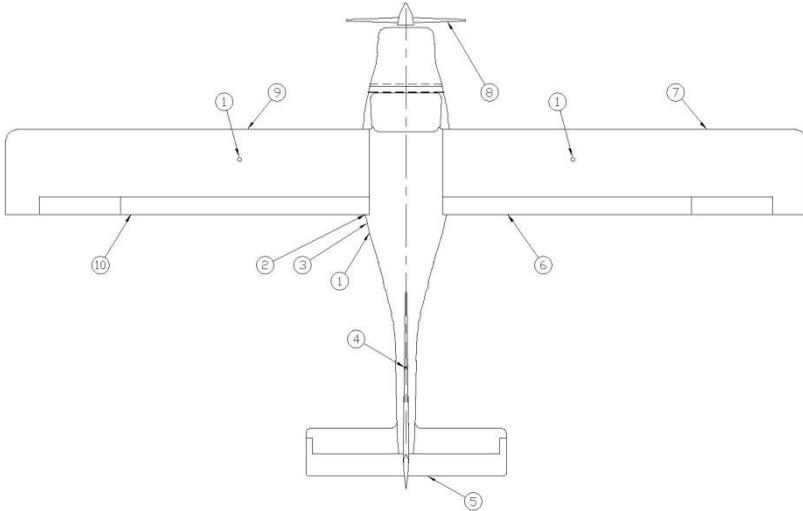
Figure 4-1. Pre-flight Inspection
