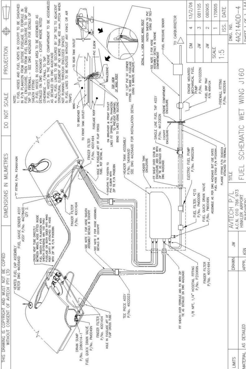
Figure 7.13 – Fuel System Schematic
