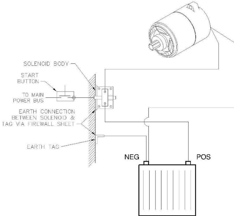
Figure 17. Starter Wiring Details
