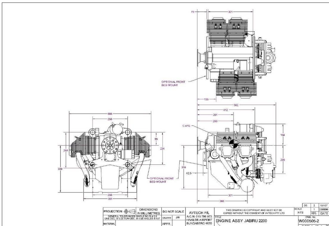
Figure 2. Drawing W00505 – Engine Dimensions S/No. 2553 On
