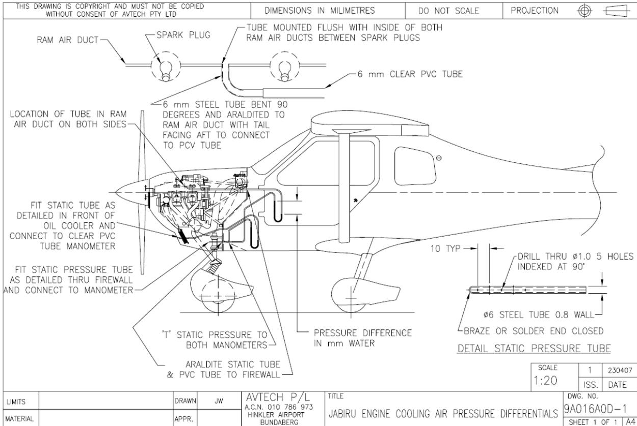
Figure 63: Cooling pressure measurement.
