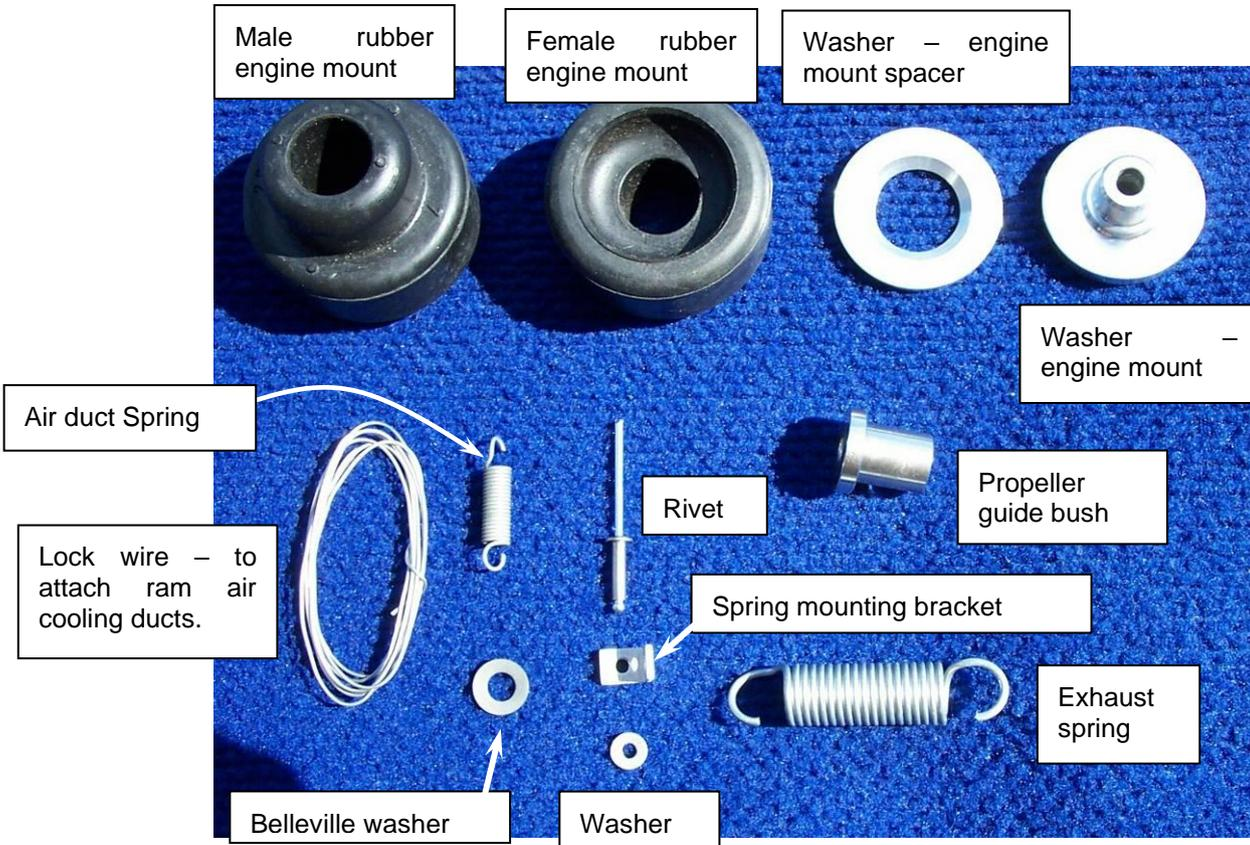
Figure 43. Engine Accessory Pack Contents
