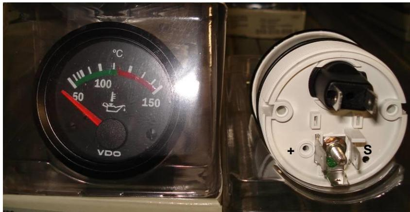
**Figure 21. Oil Temperature Connections**
