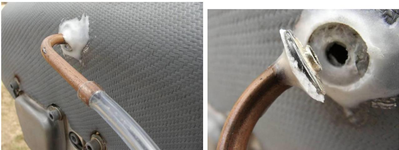
Figure 64: Ram Air duct pressure tapping.
