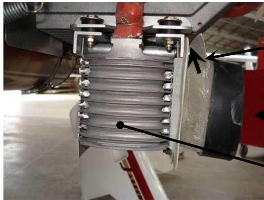
Controlled gap "leaking" air over the sump and lower parts of the engine.
