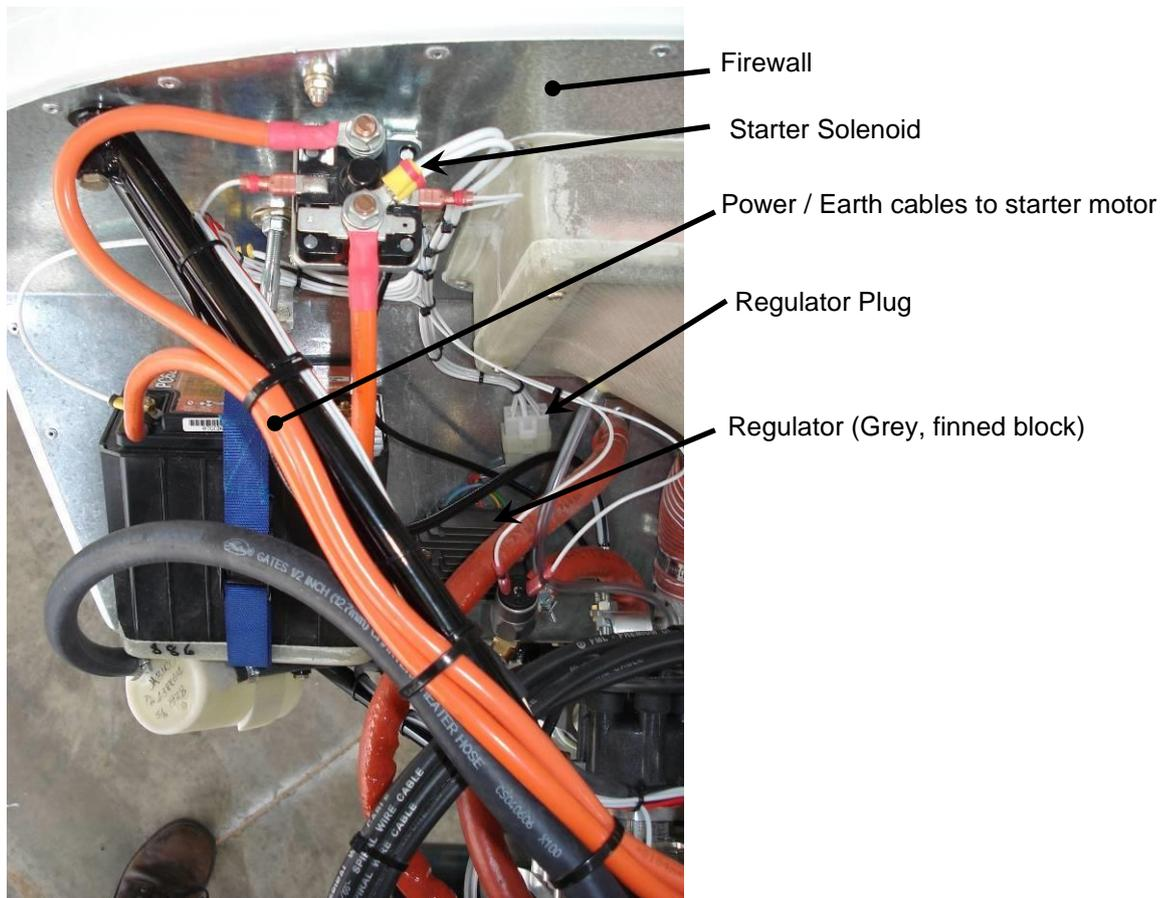
Figure 14. Electrics Installation to Firewall
