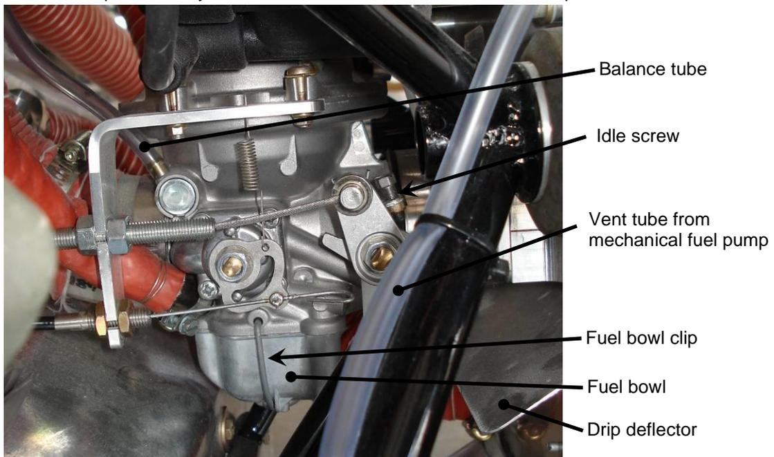
Figure 32. Carburettor Installation
