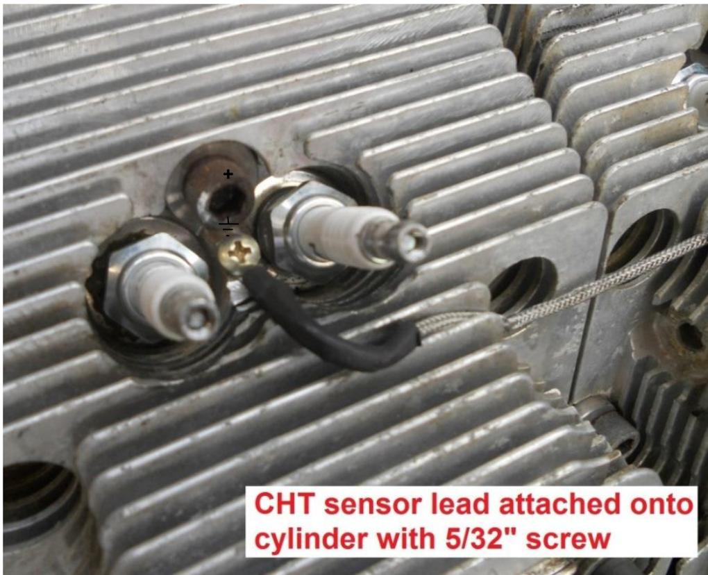
Figure 27. CHT sensor between plugs.
