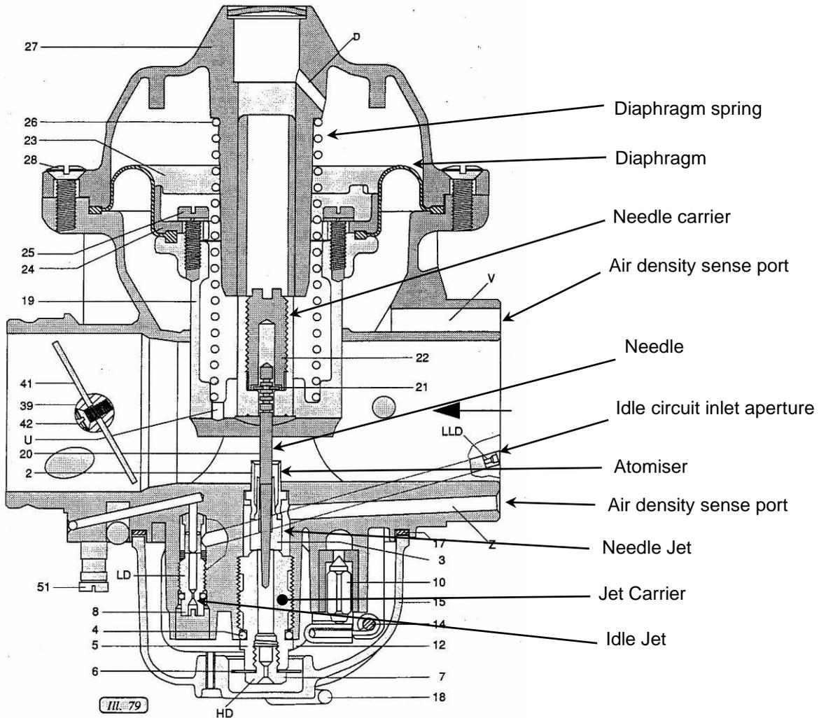
Figure 34. Carburettor Schematic
