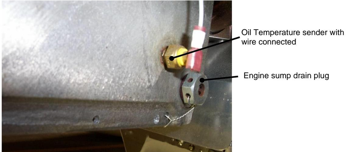
**Figure 20. Oil Temperature Sender**
