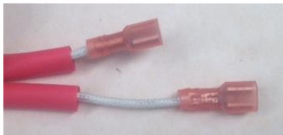
Figure 13 - Alternator leads must be of different lengths
