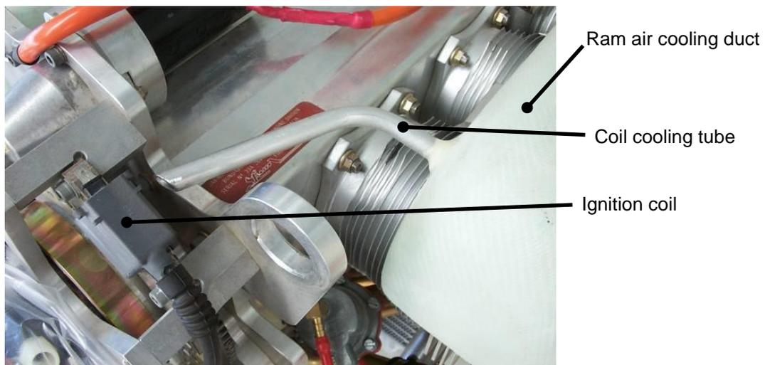
Figure 16. Ignition Coil Cooling Tube
