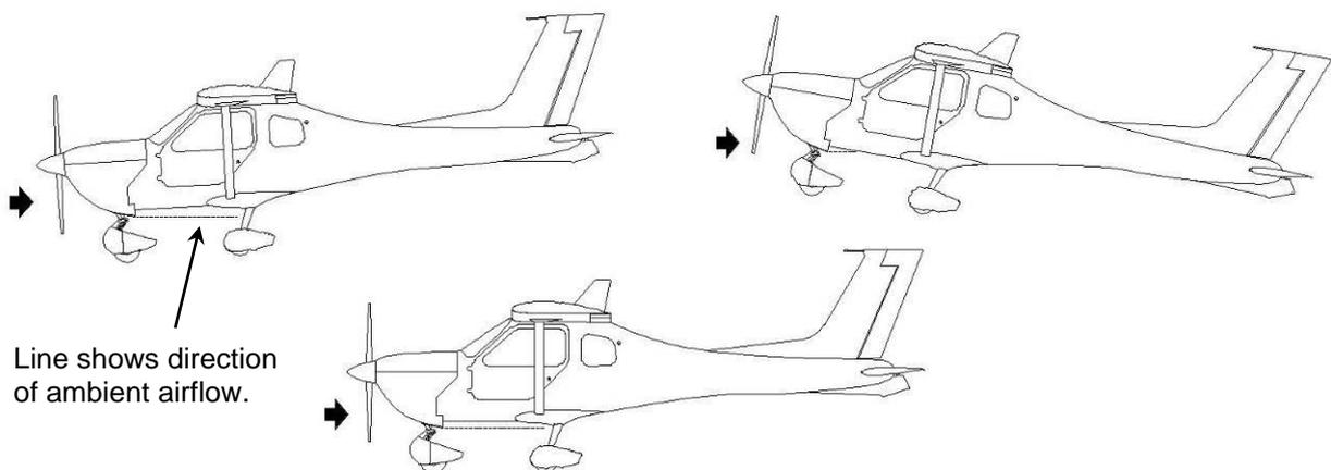
Figure 60. Affect of Angle of Attack on Cowl Outlets
