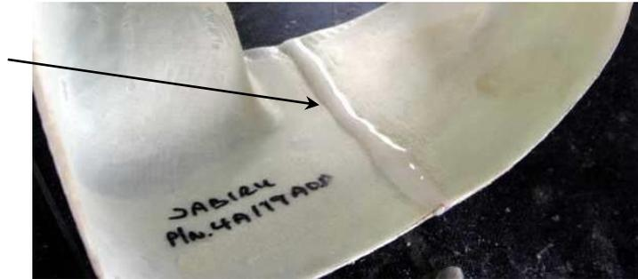
Figure 55. Ram Air Duct Front Seam
