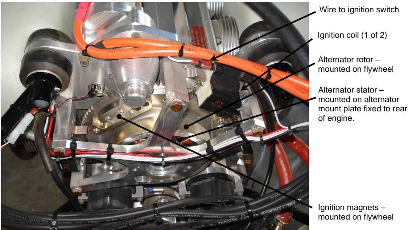
Figure 12. Ignition & Alternator Detail
