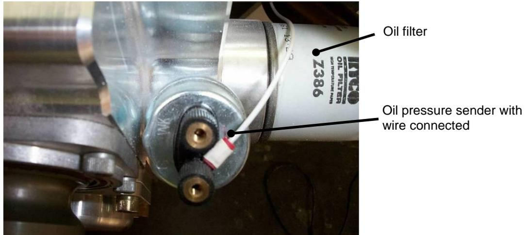
Figure 22. Oil Pressure Sender
