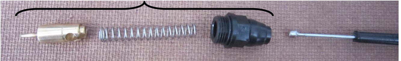
Figure 5: Choke cable end parts in order of assembly.
