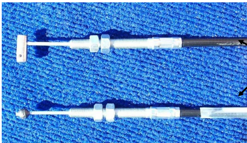
Figure 2: Throttle cable connections.
