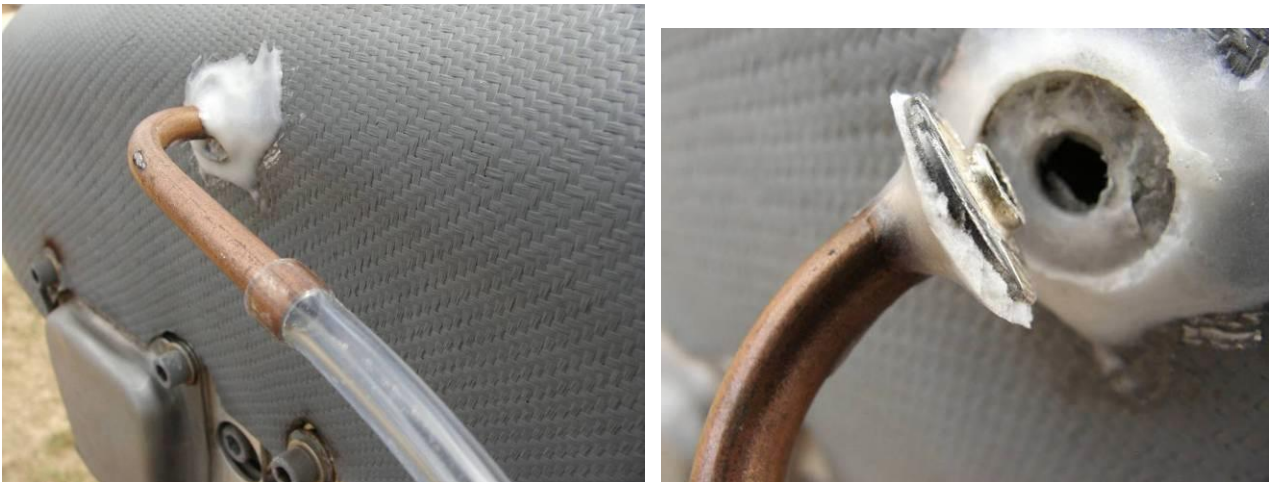
Figure 57: Ram Air duct pressure tapping.
