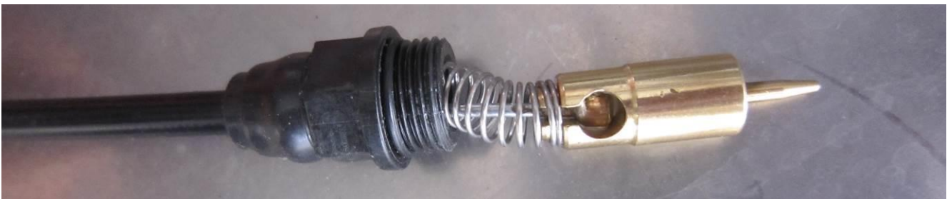
Figure 6: Choke cable end assembled.
