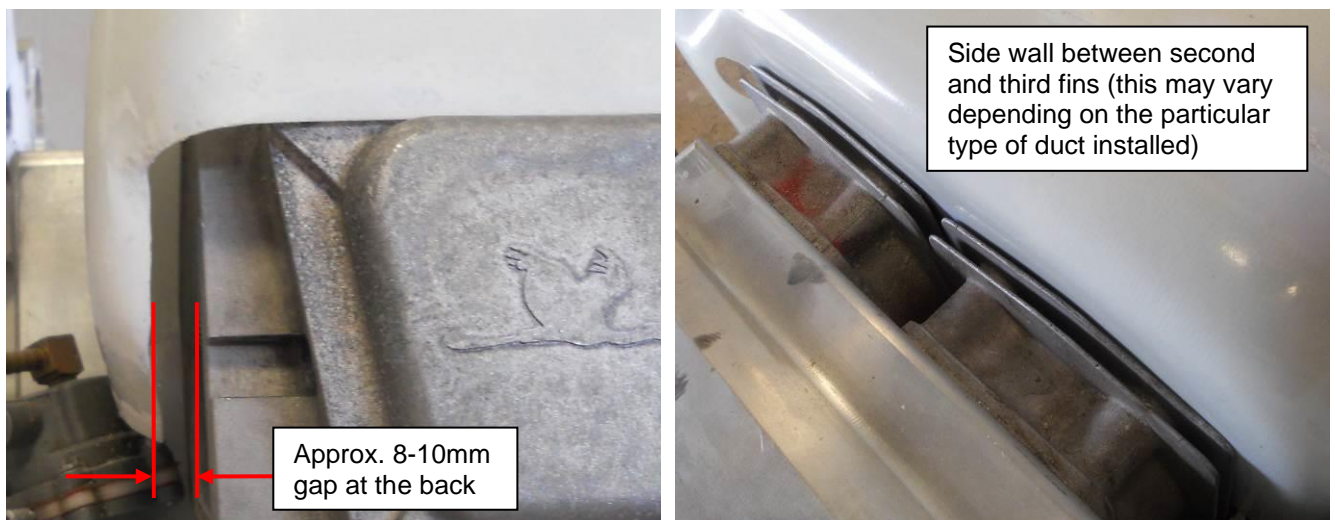
Figure 43 - Position ram-air duct on engine
