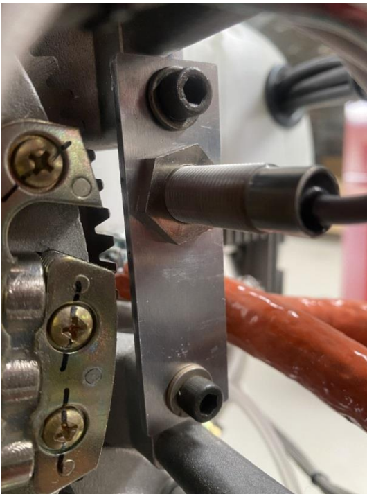
Figure 15: Hall effect sender mounting location on 3300 engine.
