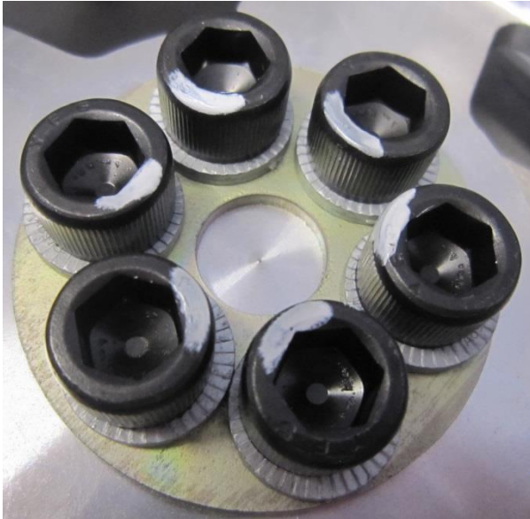
Figure 11: Flywheel bolts installed with Nordlocs and steel wear plate.
