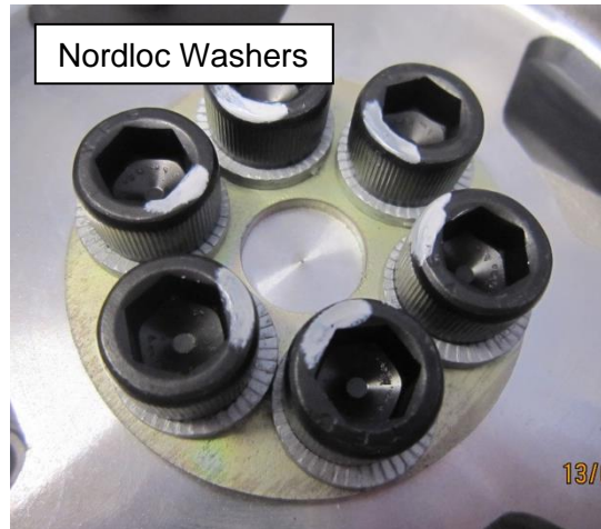
Figure 10 – Flywheel fitted with Nordloc washers
