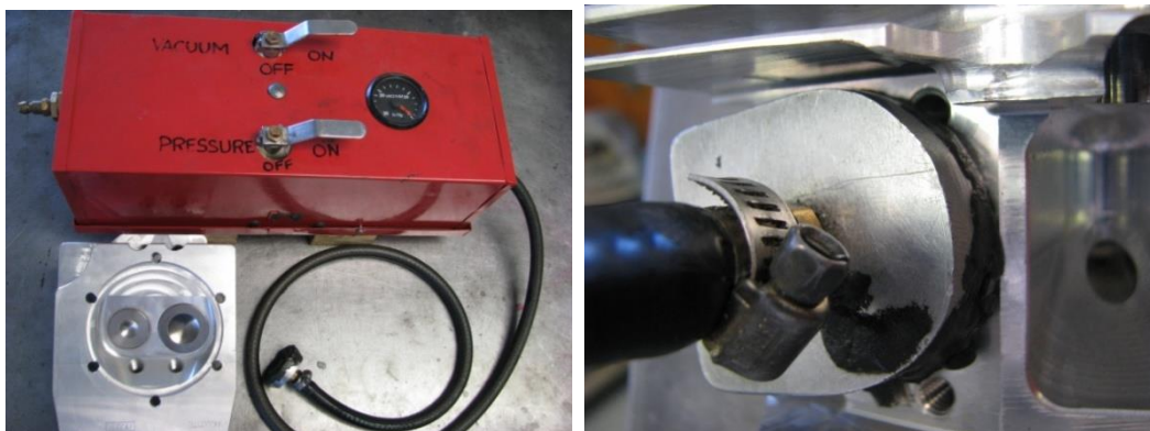
Figure 18 – Valve Leakage Vacuum Tester
