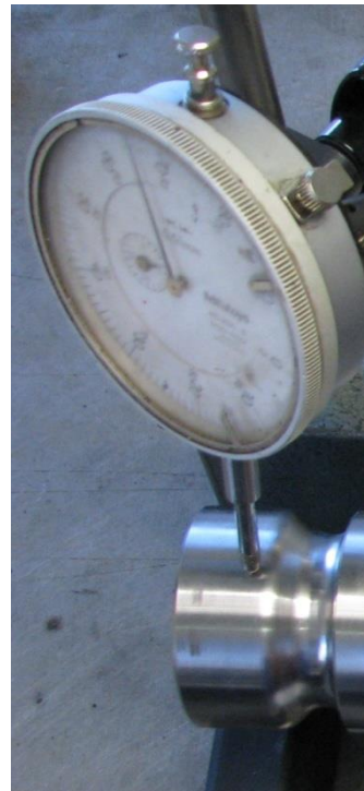
Figure 49 – Dial Indicator Position for Crankshaft & Prop Flange Run Out
