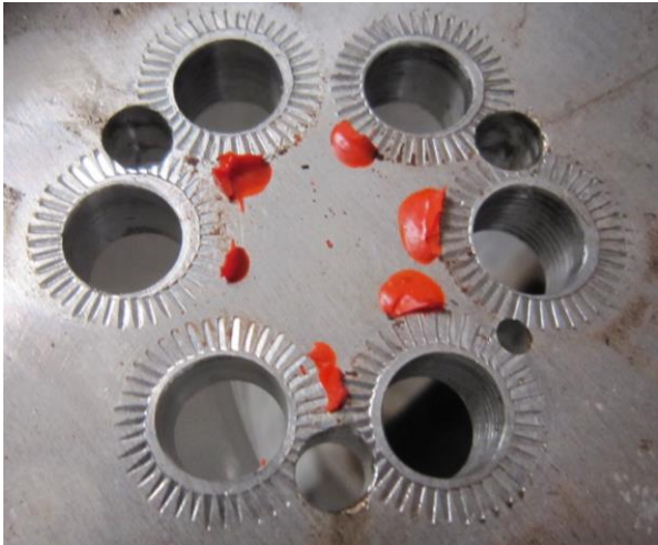
Figure 107: Indents from Nordloc washers.
