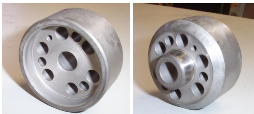
Figure 218 – Drilling Fixture – Crankshaft Side on Left, Flywheel Side On Right
