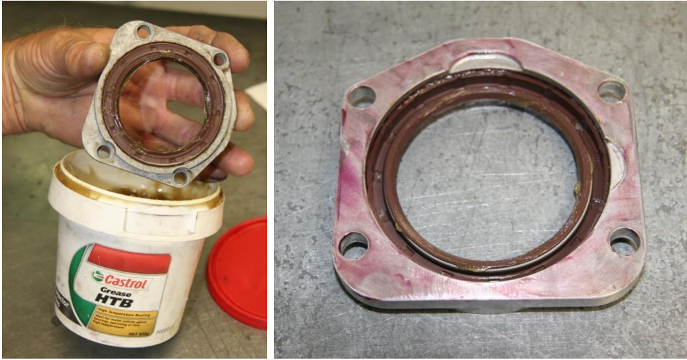
Figure 206 – Front Seal Housing Ready To Fit
