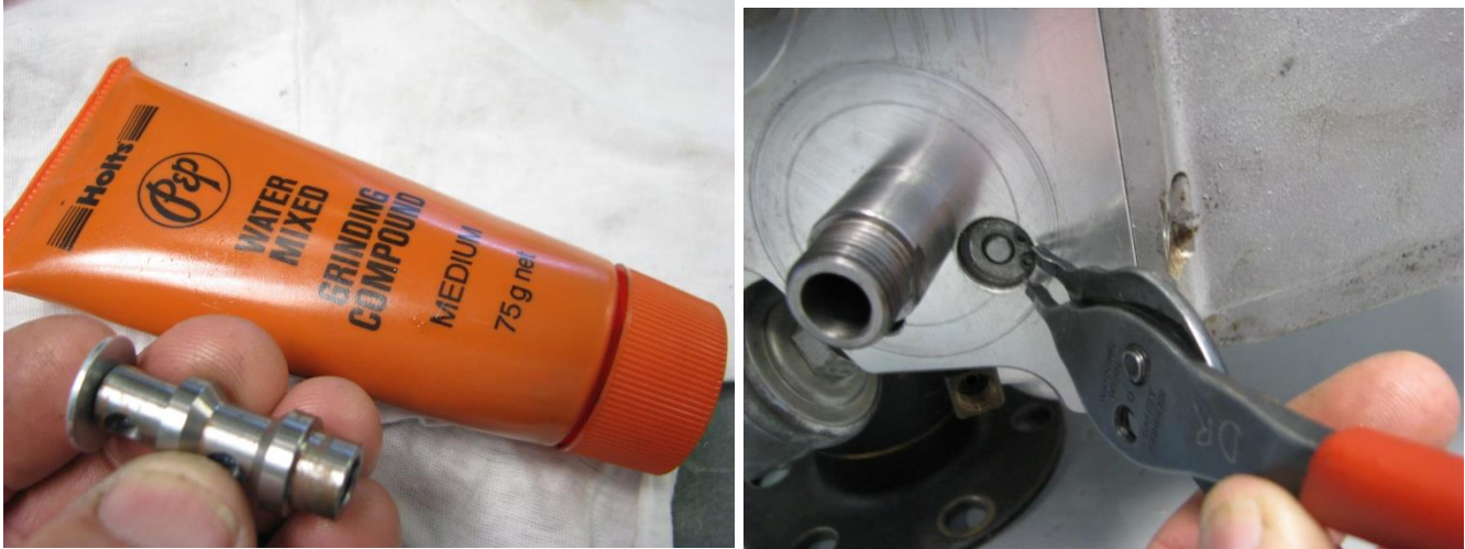
Figure 211 – Lapping Oil Pressure Relief Valve
