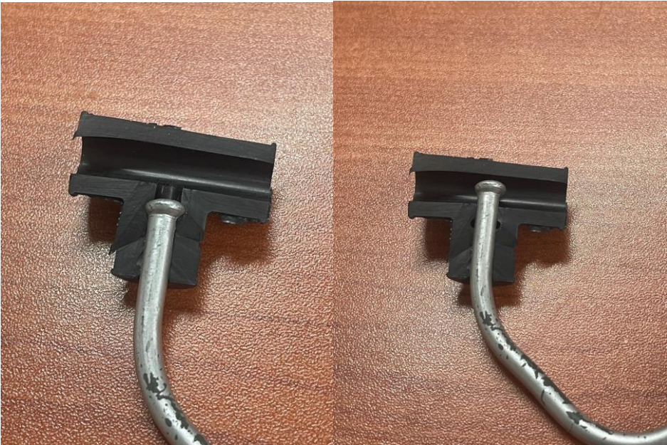
Figure 191 – Left: Correct Tube Installation in Rubber T; Right: Incorrect Tube Installation
