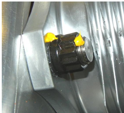
Figure 166 – Torque Seal Applied
