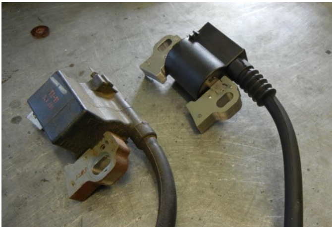
Figure 105 – Different Ignition Coil Models (Honda on Left, Jabiru on Right).
