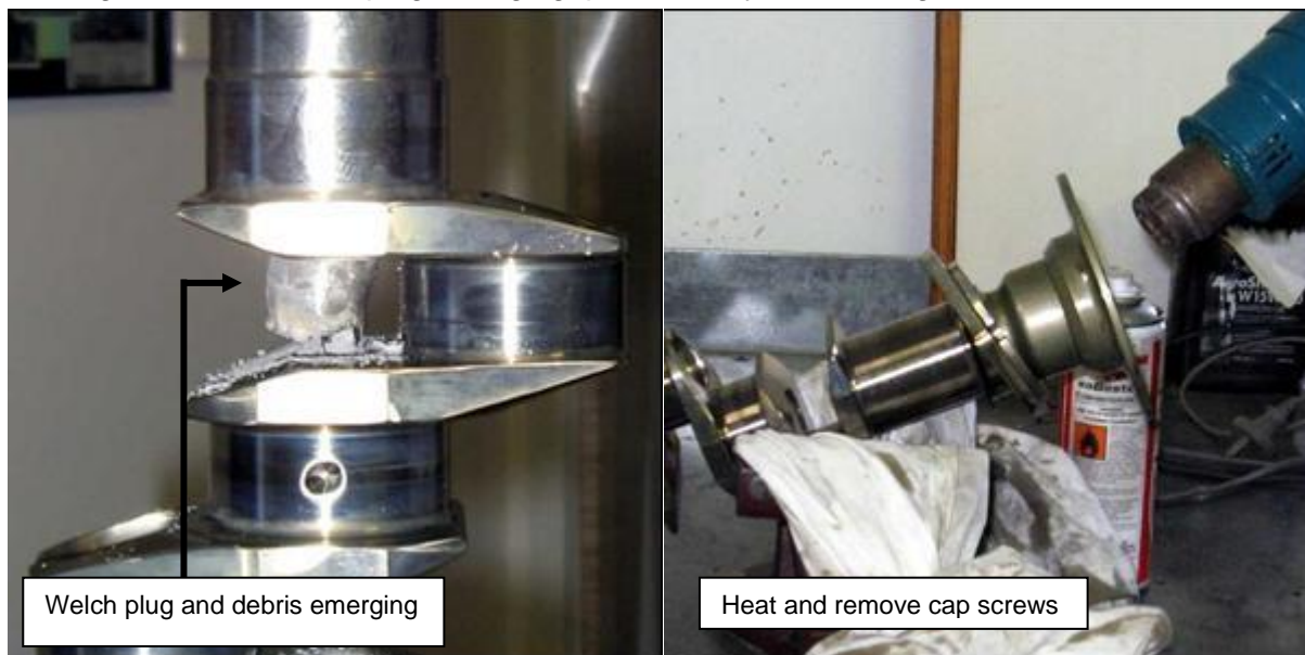
Figure 62 – Welch Plug & Propeller Flange Removal From Crankshaft
