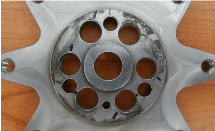
Figure 106 – Damaged Flywheel “Starfish”
