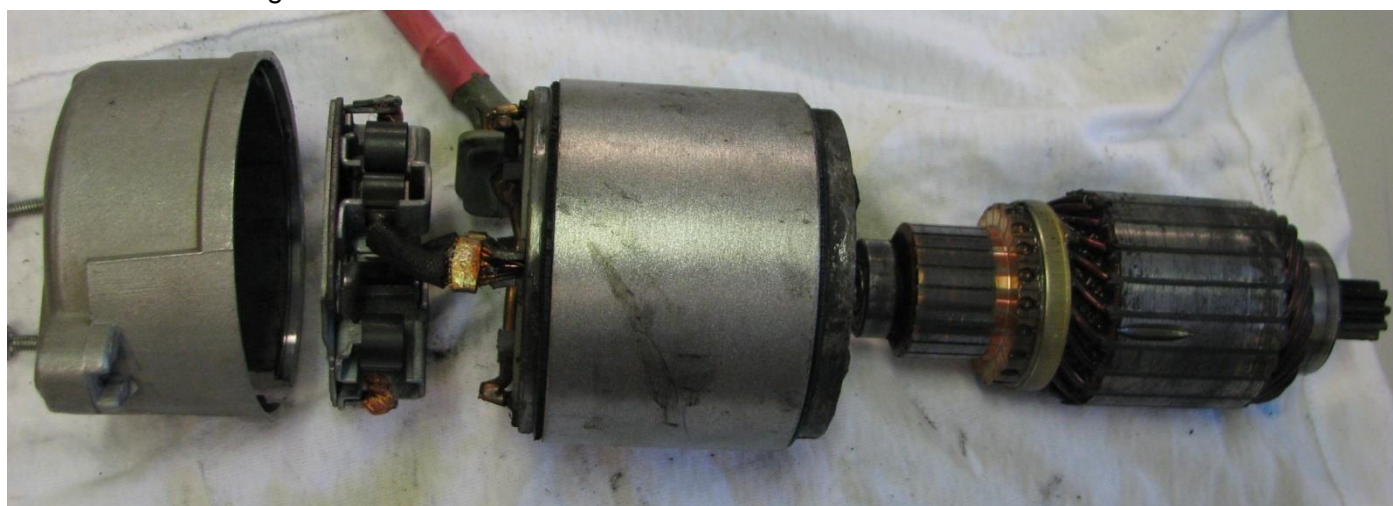
Figure 109 – Typical Disassembled Starter Motor
