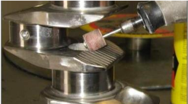
Figure 67 – Radius Crank Centre Holes
