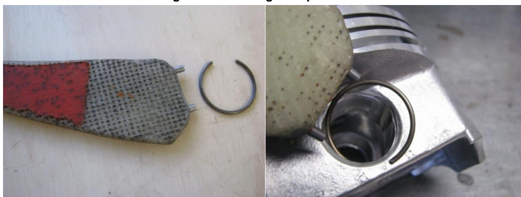
Figure 137 – Fitting Wire-Type Piston Circlips
