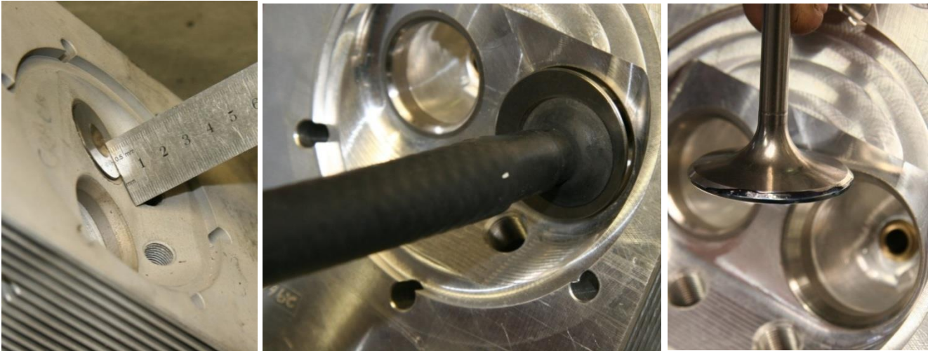
Figure 95 – Recessed Valve Seat, Valve Being Cut
