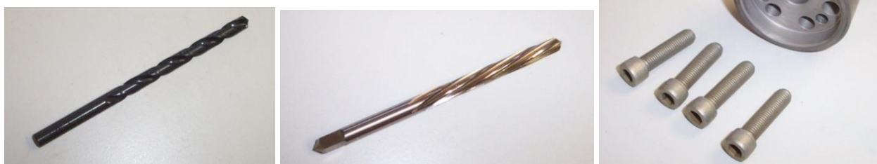
Figure 219 – 15/64” Drill (Left), 6mm Ream (Centre), UNF Cap Screws (Right)
