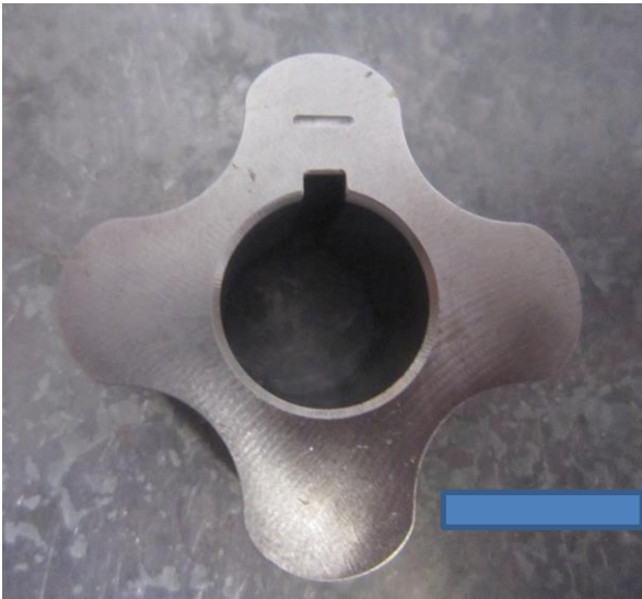
Figure 82: Broad lobe inner gear with line marking.
