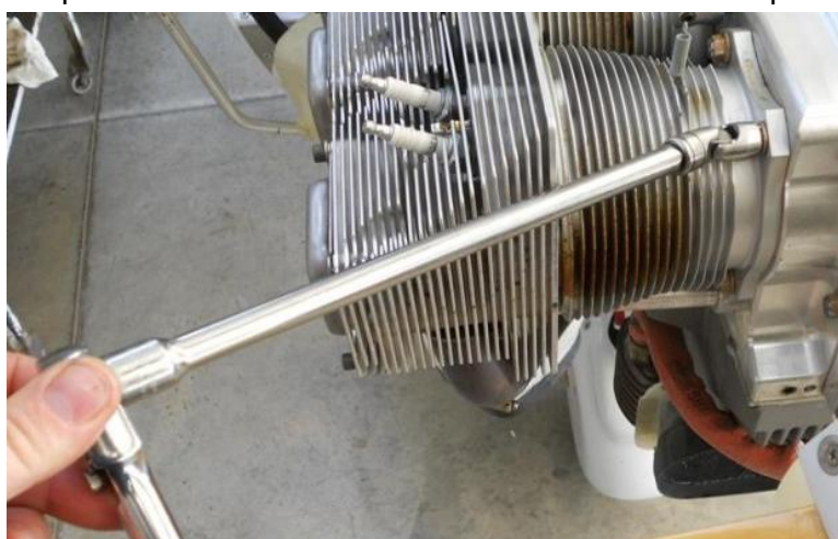
Figure 167 – Universal Joint tool FU14B (FU16B for 1/2" Socket)
