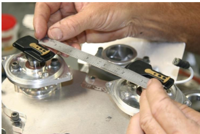
Figure 180 – Checking Rotors, Tightening Distributor Case
