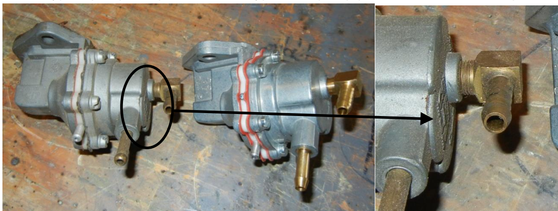
Figure 120 – Fuel Pumps (Type 1 on Left, Type 2 on Right)
