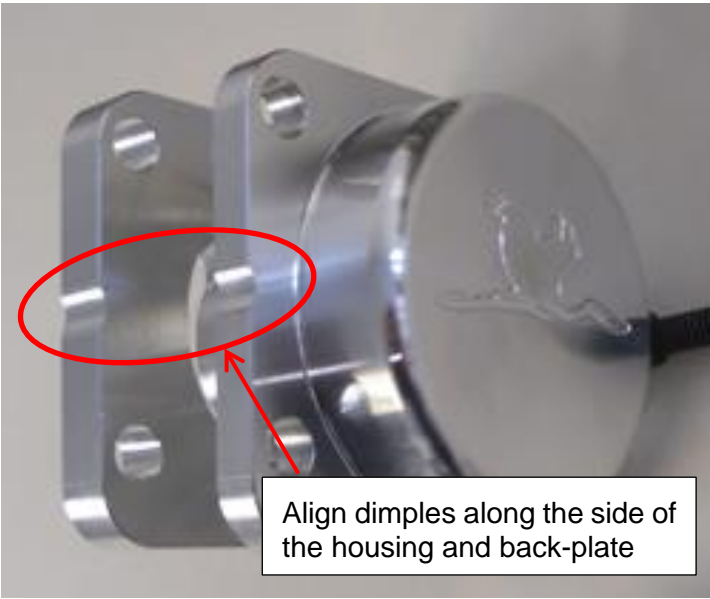
Figure 84 - Oil pump housing and back-plate alignment (six-lobe pump)
