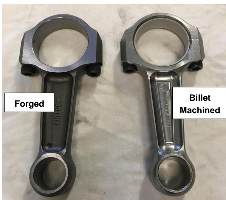
Figure 125 - Forged conrods vs Billet machined conrods
