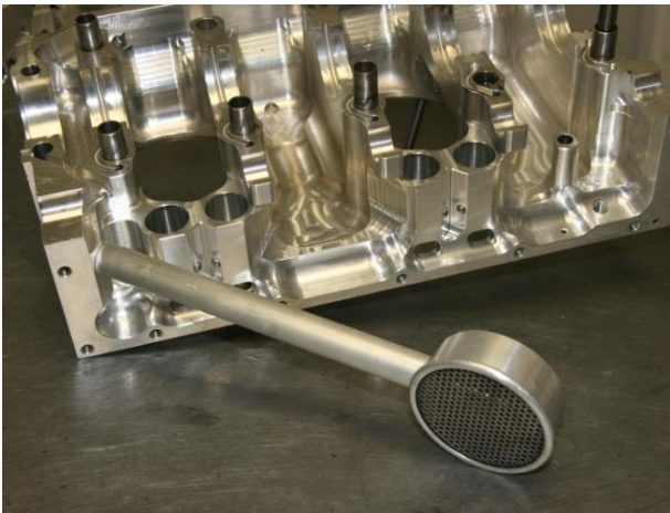
Figure 130 – Fitting Oil Pickup Tube
