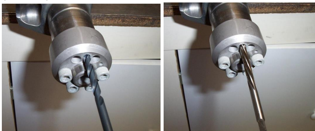
Figure 221 – Drilling & Reaming Crankshaft – ILLUSTRATION ONLY.
